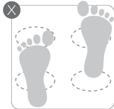
The feet are too far apart or close to the edge, resulting in inaccurate measurements.
