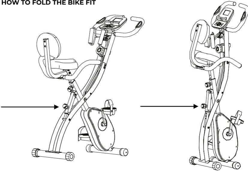
1. Pull out the ball pin into the position.
